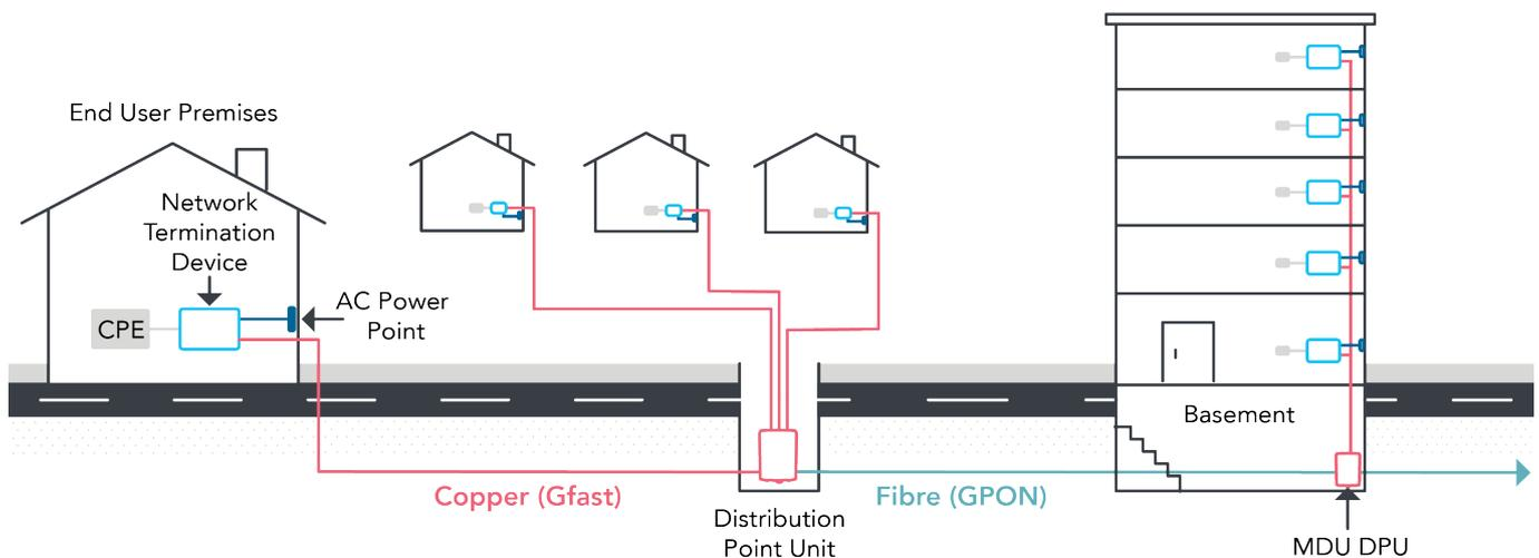
To streamline deployment, the DPU can be installed without activating any of the end-users. The DPU can have a built-in POTS bypass which means that if the end-user doesn't sign up for the service (there is no NTD connected), the end-user remains connected to the traditional legacy xDSL service coming from the central office or cabinet. Once the end-user self-installs the NTD, the higher-speed Gfast service is turned on and the end-user can benefit from high-speed broadband.
